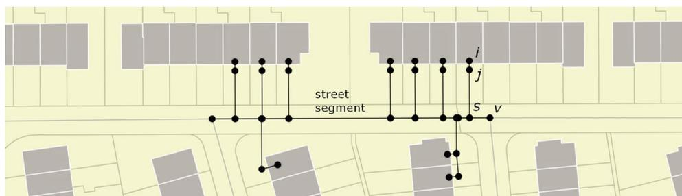
Fig. 2. Nodes of a hypothetical heating grid.
